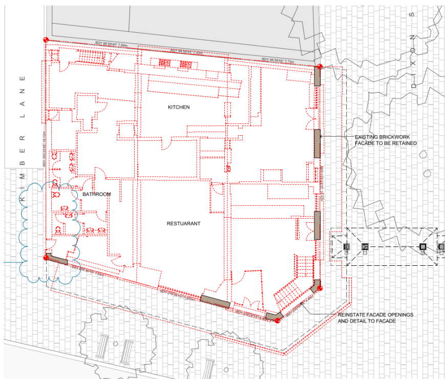
Figure 8: indicative demolition plan (ground level)
